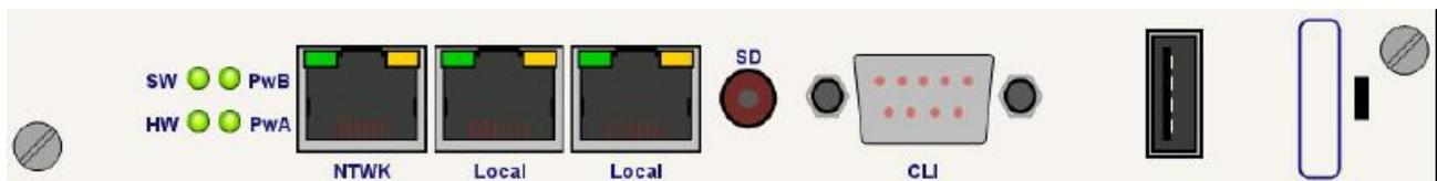
The management MGNT4 board is used to connect the equipment to the network and to make it manageable remotely through web based http craft terminal. It supplies the applications allowing to communicate with the boards inserted in the chassis and to configure them.
