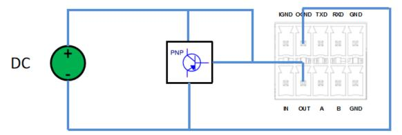
OUT corresponds to OUT on 2\*5 3.5mm interface, and OGND corresponds to OGND on 2\*5 3.5mm interface. The
