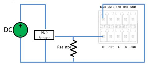
IN corresponds to IN on 2\*5 3.5mm interface, and IGND corresponds to IGND on 2\*5 3.5mm interface. The voltage range of external power supply (DC) is  $3V \sim 30V$ ; the internal flow of the device is limited. In the normal voltage range, the external power supply does not need to be limited.
