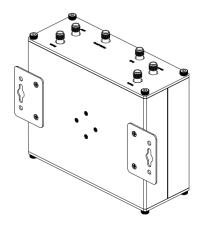
Use 4 pcs of M2.5\*4 flat head Phillips screws to fix the wall mounting kit to the router, and then use 2 pcs of M3 drywall screws to mount the router associated with the wall mounting kit on the wall.
