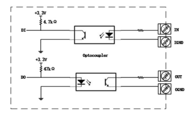
The MS659100M supports 1 channel DI and 1 channel DO by default. It can support 2 channels of DI or 2 channels of DO by BOM modification. DI signal access, can be used for NPN/PNP type sensor signal or switch signal acquisition, power supply can only be accessed from IN, not reversed. DO signal output, can be used for NPN/PNP sensor control.
