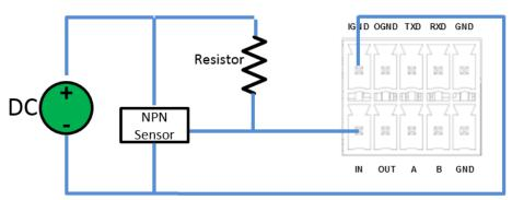
IN corresponds to IN on 2\*5 3.5mm interface, and IGND corresponds to IGND on 2\*5 3.5mm interface. The voltage range of external power supply (DC) is  $3V \sim 30V$ . The internal flow of the device is limited. In the normal voltage range, the external power supply does not need to be limited.
