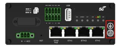
Router grounding helps prevent the noise effect due to electromagnetic interference (EMI). Connect the router to the site ground wire by the ground screw before powering on.
