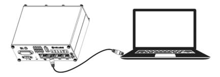
Connect an Ethernet cable to the port marked ETH1~ETH3 at the front of the MS659100M Router, and connect the other end of the cable to your computer.
