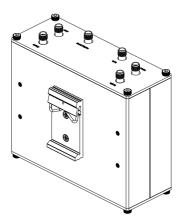
Use 2 pcs of M3\*6 stainless flat head Phillips screws to fix the DIN rail to the router, and then hang the DIN rail on the mounting bracket. It is necessary to choose a standard bracket.
