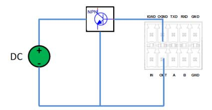
OUT corresponds to OUT on 2\*5 3.5mm interface, and OGND corresponds to OGND on 2\*5 3.5mm interface. The maximum 2.5mA drive current can be supplied through OGND; the external power supply DC voltage range is 3V~30V.
