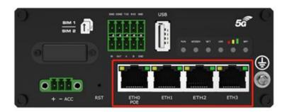
There are four Ethernet ports on MS659100M, including ETH0 (POE), ETH1, ETH2, ETH3. Each has two LED indicators. The yellow one is a link indicator but the green one doesn't mean anything. For details about status, see the table below.
