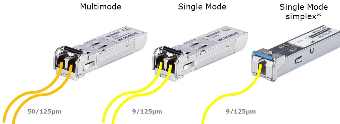
\* Attention: for simplex (fiber-optic or bi-directional communication), make sure that the appropriate wavelengths are used (TX/RX transmit and receive direction) and that the transceivers are used in pairs (A<->B).
