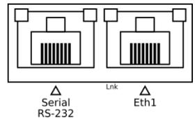
Fig. 3: Port status LEDs
