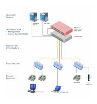
Network with decentralised switching architecture and centralized network access control.
