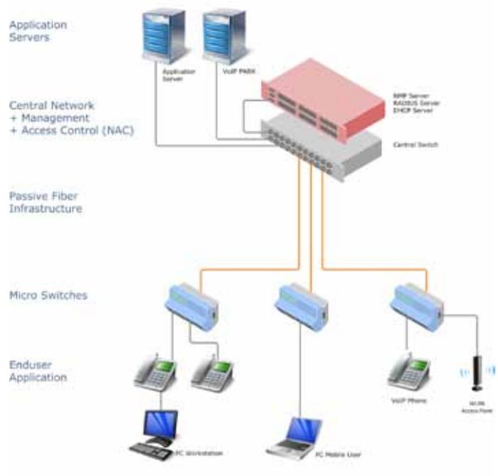
Network with decentralised switching architecture and centralized network access control.
