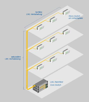
Fiber optic-based network topologies such as FTTO, use cabling with an extremely long product life cycle and a maximum of performance capacity.
